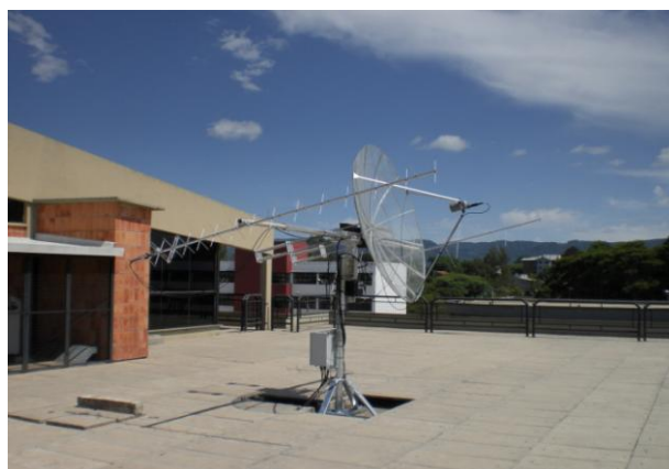
Fig. 9: The NANOSATC-BR's Ground Station (GS) with VHF/UHF band and S-band antennas at CRS/CCR/INPE-MCTI, in Santa Maria, RS.
